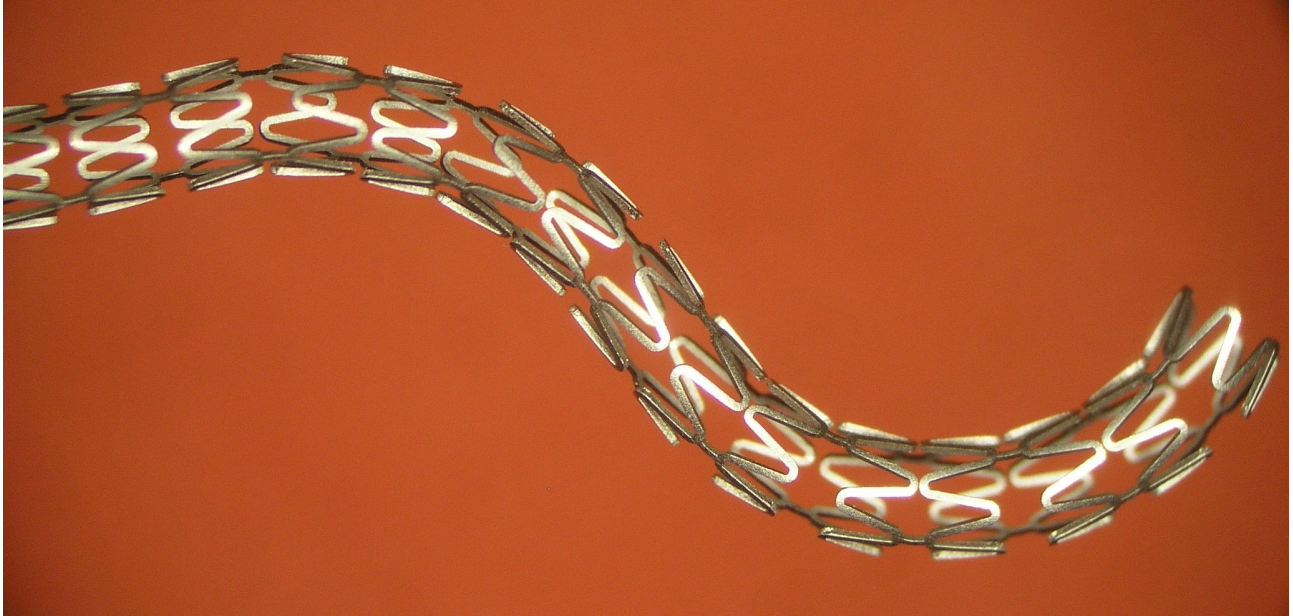
Picture 4.: Flexibility of FMC23 Stent (before polishing)
